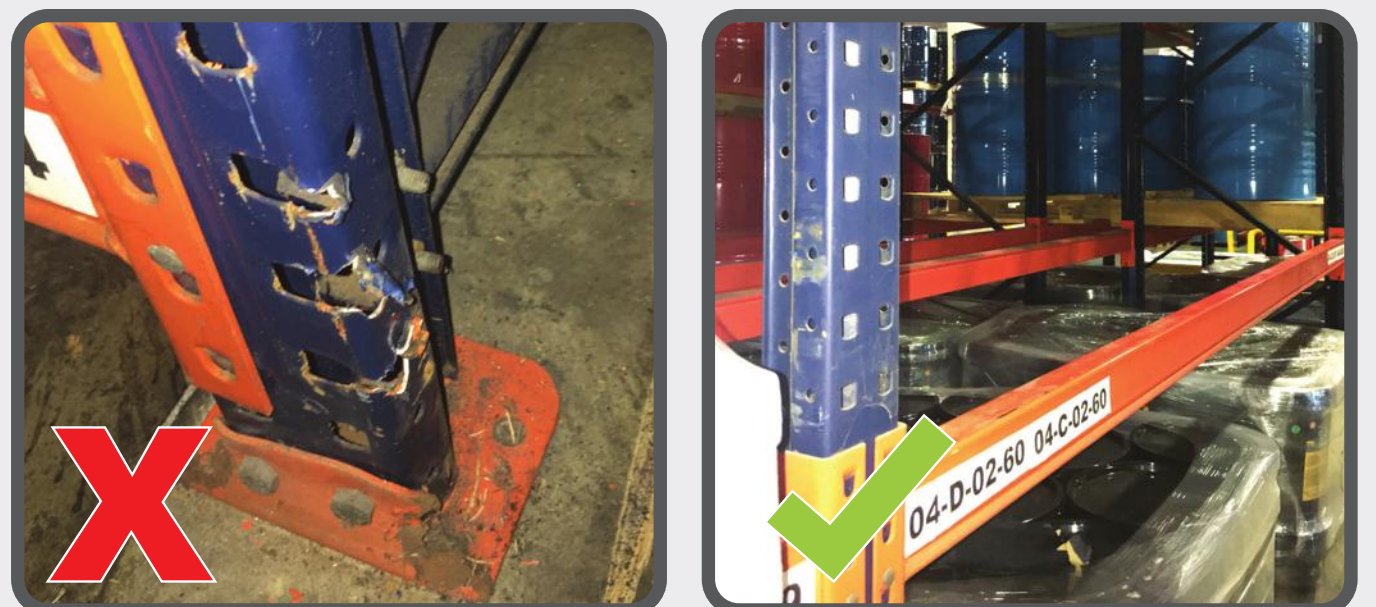
Report damaged racks and avoid using them
